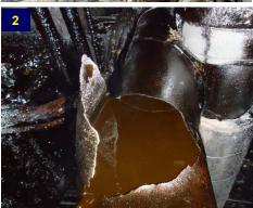
In both of these incidents, the Mechanical Integrity Management System was not successful in detecting or replacing deteriorated piping components before failure. In the 2013 incident, the maintenance system did not ensure that the correct material of construction was used when the pipe was replaced. More effective mechanical integrity and maintenance programs could have prevented both incidents.
