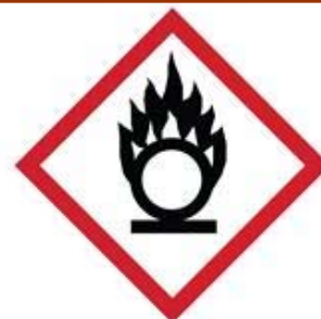
The symbol for an oxidizer in the United Nations "Globally Harmonized System of Classification and Labeling of Chemicals" (adopted by US OSHA in May 2012)
