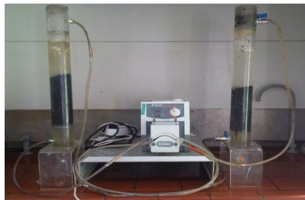
Figure 2. The granular activated carbon submerged up-flow reactors, (a) nitrification column and (b) denitrification column
