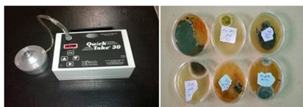
Fig. 1. Airborne fungal spores plates and related air sampling equipment's
