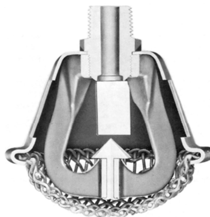
FIGURE A.3.3.6.4 Foam-Water Spray Nozzle.
