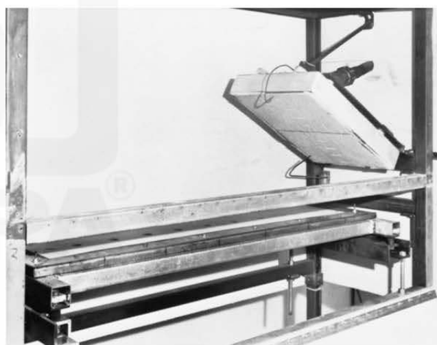
FIGURE 4.1(b) Flooring Radiant Panel Test Apparatus Showing Carpet Specimen and Gas-Fueled Panel.
