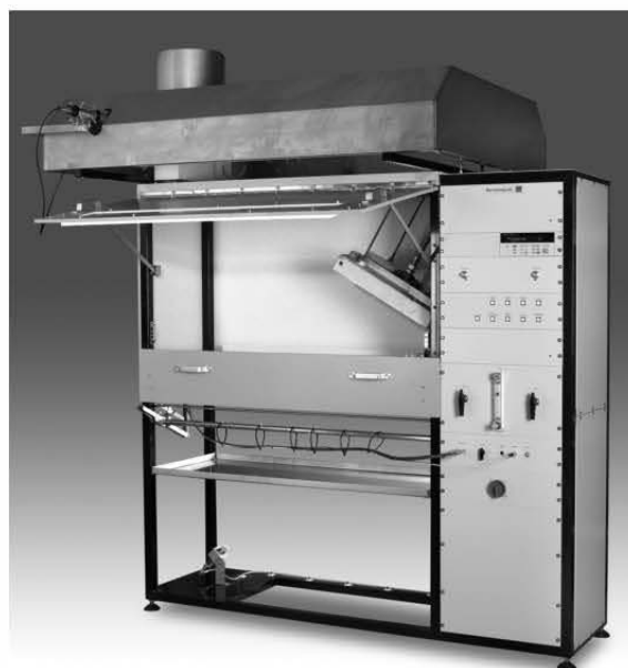
FIGURE 4.1(a) Flooring Radiant Panel Test Apparatus.
