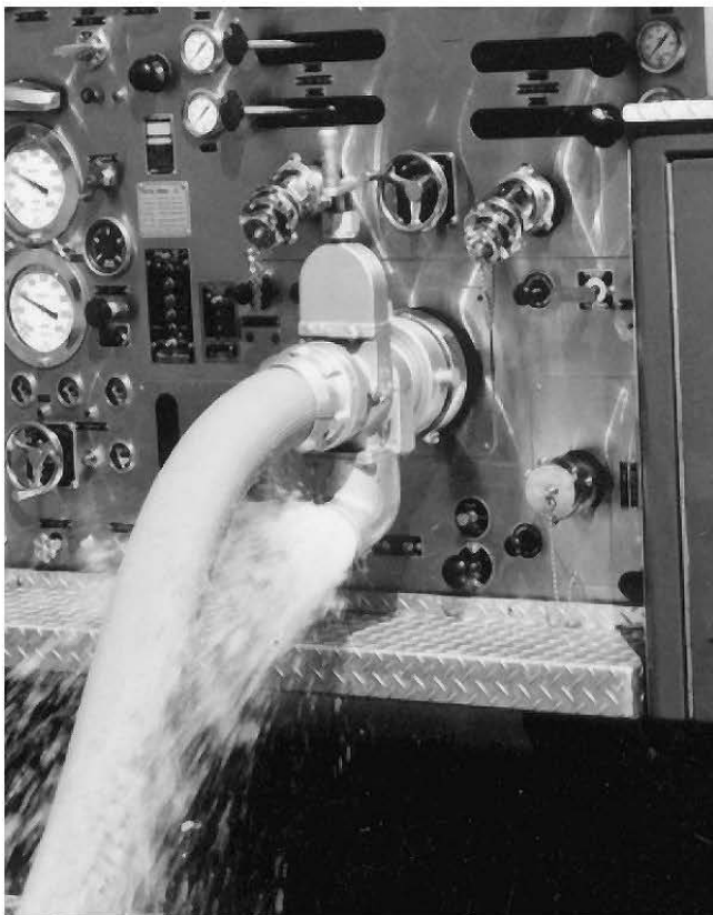
FIGURE D.5.4 Intake Gated Relief Valve.
