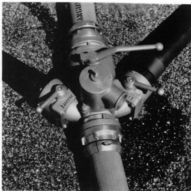
Figure D-1.7.5 Distributor valve.
